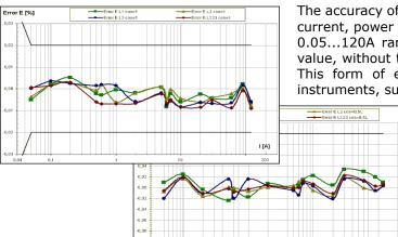
The accuracy of the basic parameters of the Calmet TB10 - voltage, current, power and energy in a wide voltage 21...560V and current 0.05...120A ranges, is expressed as a percentage of the setting value, without the component as a percentage of the range value. This form of errors specification is very useful when checking instruments, such as electricity meters.
