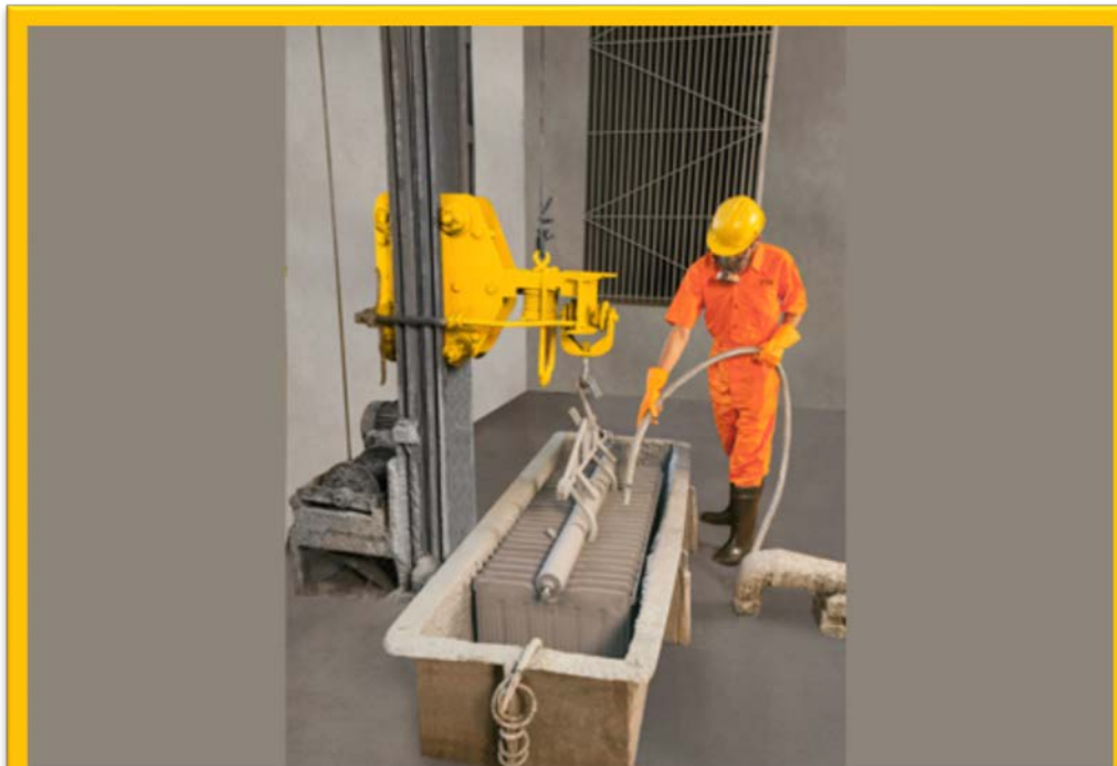
4.0 meter deep, paint flooding tank
