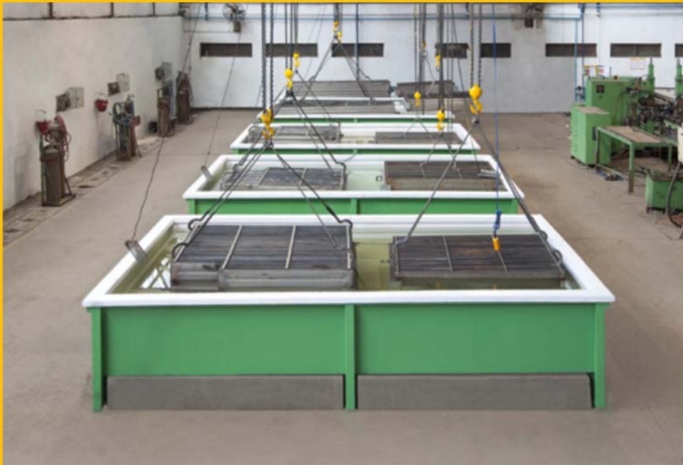
Radiator testing tanks
