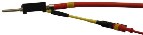
safety voltage cables in order to furnish phase voltages with using safety crocodile test clip.
