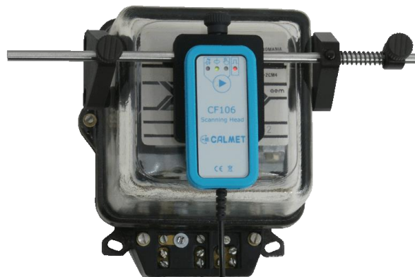
Test of electricity meter with rotor (scanning head mounted by using holder – CF106H option)
