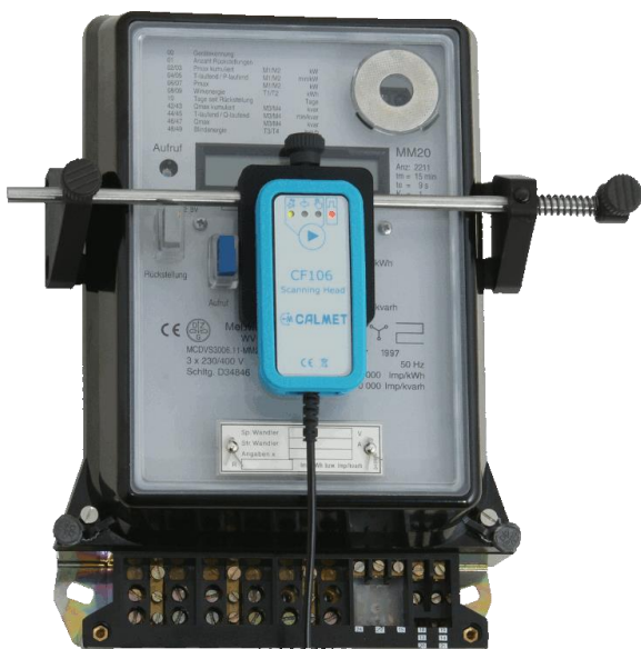
Test of electricity meter with LED (scanning head mounted by using holder – CF106H option)
