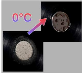
indicate the precise moment at which the ice melts. The 973-SF<sub>6</sub> measures the actual mirror temperature at that very moment and provides a pass/fail indication.
